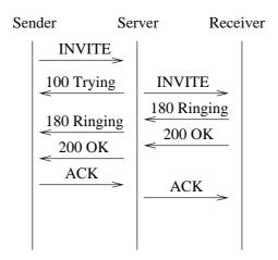
Figure 2: Illustration of a sender initiating a call with a receiver. It is assumed that both the sender and receiver have registered with the server before this.
