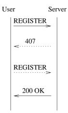
Figure 1: Illustration of a user registering with a server. A non authenticated register includes only the solid line messages; an authenticated register includes both solid and dotted line messages.
