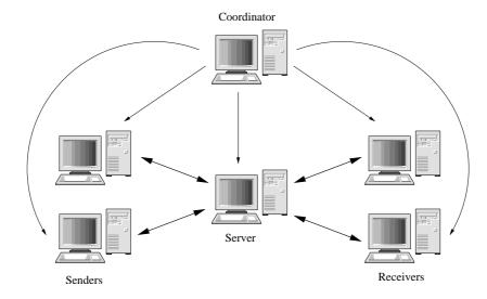
Figure 3: The experimental setup. The bold lines indicate SIP traffic, the regular lines indicate coordination information.
