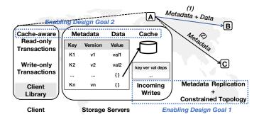
Fig. 3: The system architecture of K2. Each datacenter has the entire keyspace sharded across servers, and a small amount of cache. It stores data for a subset of keys and only metadata for the rest. K2 partially replicates data and fully replicates metadata by following a constrained topology.
